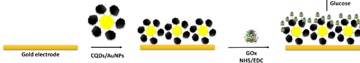
Figure1: schematic representation of the overall biosensor and chronoamperometric response of the developed biosensor to the serial additions of glucose under stirring conditions, applied potential: -0.6V.
